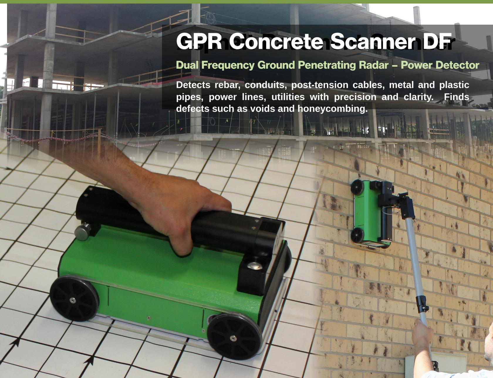
The ESS Concrete Scanner DF has been designed to detect deep subsurface targets while still providing high-resolution. The dual frequency antennas produce high-resolution scans without sacrificing penetration depth. The 2 GHz antennas sense objects to about 2 feet depth, while the 750 MHz sensors detect objects as deep as 4 feet.
