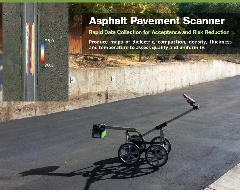
The **Asphalt Pavement Scanner** continuously measures dielectric using advanced radar technology with additional integrated sensors. An optional calibration process converts dielectric to density and compaction. The integrated **precision GPS receiver** allows **detailed maps of density, compaction and temperature** to be generated with centimeter-level resolution. Cart-mounted
