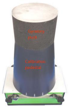
The **Asphalt Mix Calibration Kit** is an accessory to the Asphalt Pavement Scanner (APS) that provides the asphalt mix specific calibrations. Starting with a set of gyratory compactor pucks, the dielectric constant of each puck is measured using advanced radar technology. Then the density of each pucks is determined using a water displacement method such as AASHTO 166. The APS software creates a mix calibration that can be transferred to scanners operating at the job site.
