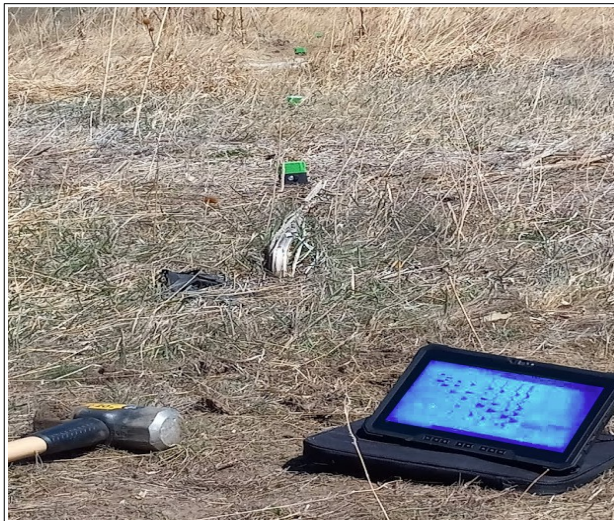
Figure 1: The Cube Seismic system includes eight wireless seismometers (green boxes) mounted on eight-inch spikes and a tablet equipped with software for data processing and viewing. The 20 lb. sledgehammer used in this survey (shown) was provided by the user.
